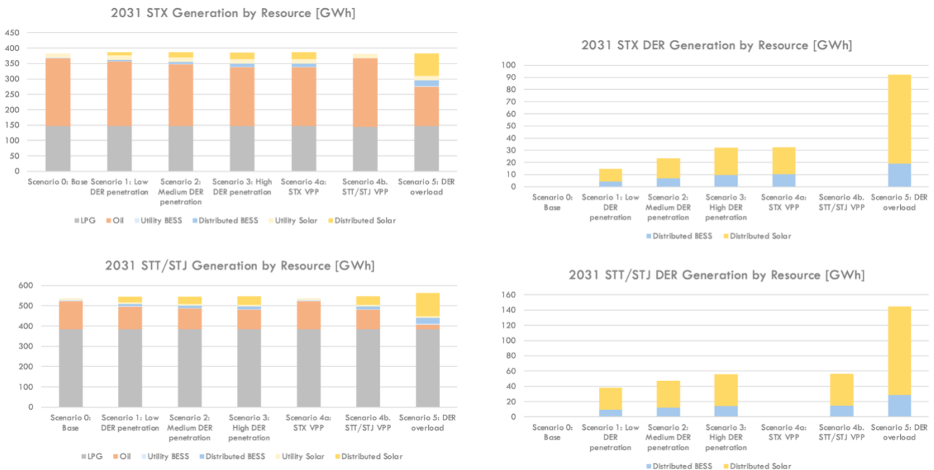
Figure C.10-Annual STX generation [MWh] (upper left), annual STX DER generation [MWh] (upper right), annual STT/STJ generation [MWh] (lower left), annual STT/STJ DER generation [MWh] (lower right) by resource and scenario
