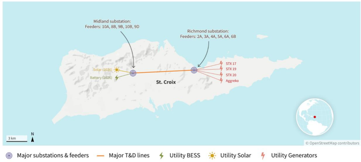
Figure 10 - Simplified grid topology for the St. Croix grid used in the VPP PLEXOS analysis.
