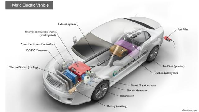
Figure 2. Hybrid Electric Vehicle (HEV).
