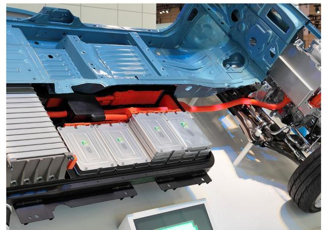
Figure 3. Nissan LEAF® cutaway showing part of the battery.
