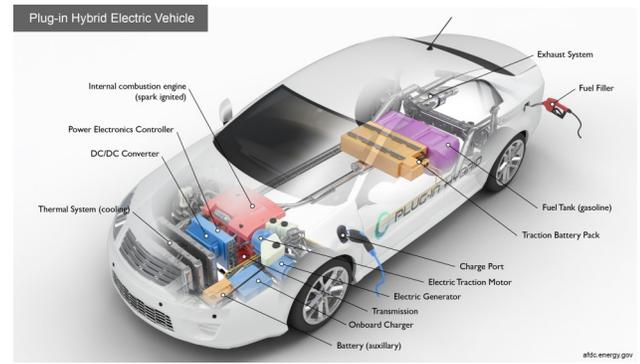
Figure 1. Plug-In Hybrid Electric Vehicle (PHEV).
