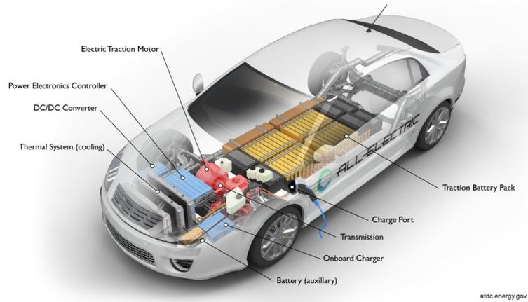
**Figure 4. Diagram of All-Electric Vehicle components.**
